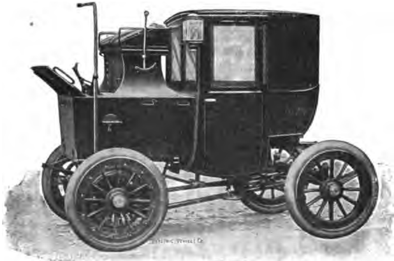
FIG. 59. —Front-Driving Brougham of the Electric Vehicle Co., used in New York City. This model, which is no longer manufactured, represents a construction very suitable for city service, but quite inappropriate for country and general use.
